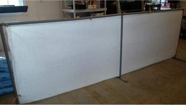
Lightweight court dividers –made of  $\frac{3}{4}$ " PVC electrical conduit, tees, elbows and tarp. Cost was ~ \$20 per panel.
